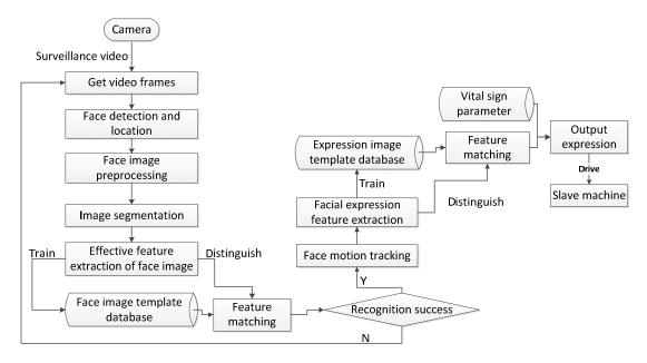
Figure 1 flow chart of face recognition system
